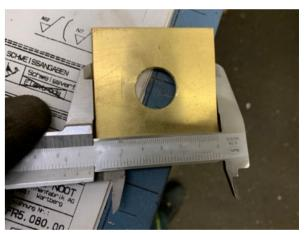
When you have one Measurement correct between 2 Edges continue with the last Edge.
