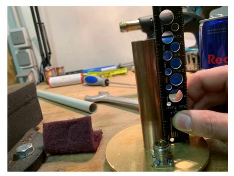
Wrap some Aardboard or thick Paper around the Tube and put it into the vice as shown on the Picture. Its recommended that you lay the Reflector onto the Jaws of the Vice so everything keeps in Place even when the Reflector gets bigger due to the Heat.
