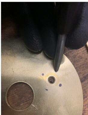
Put the M3 Threadcutter into the Powerdrill and switch the speed as Low as possible.
