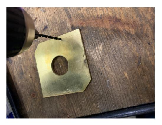
Use a Countersink or a larger Drill to deburr the Hole on both Sides.
